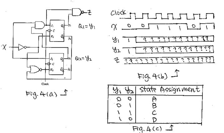
5. (18%) A Moore sequential circuit has one input, X, and one output Z. When the input sequence 011 occurs, the output becomes 1 and remains 1 until the sequence 011 occurs again in which case the output returns to 0. The output then remains 0 until 011 occurs a third time, etc. For example, the input sequence
